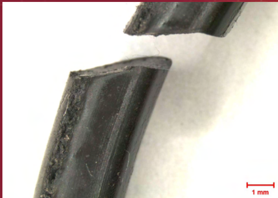
Image showing the complete failure of an O-Ring and surface damage extending around the circumference.
