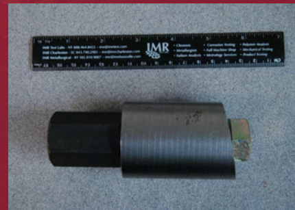
Intact bolt in 10 degree wedge fixture
