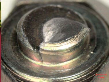
As received and macroscopic views of failed fastener sample
