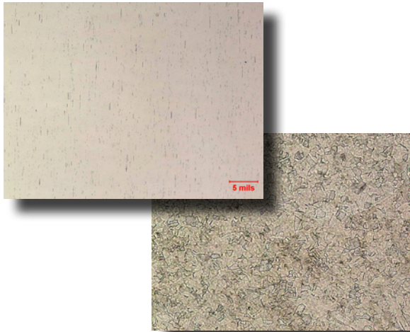
Inclusion Rating and Grain Size of a fastener as polished 100x
