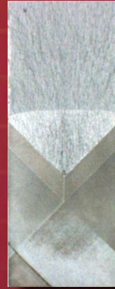
Fracture Mechanics Specimens after Fatigue Pre-cracking and K1c Testing
