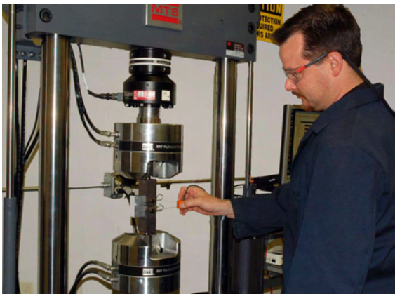
Director of Materials & Product Testing, Bill DeLaurier, setting up a fatigue sample.
