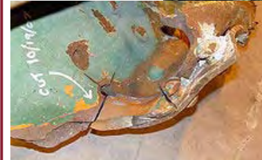
Broken Gusset Plate from Bridge Failure
