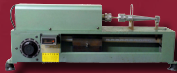
Rotating Beam Fatigue with High Temp Capability to 1800F
