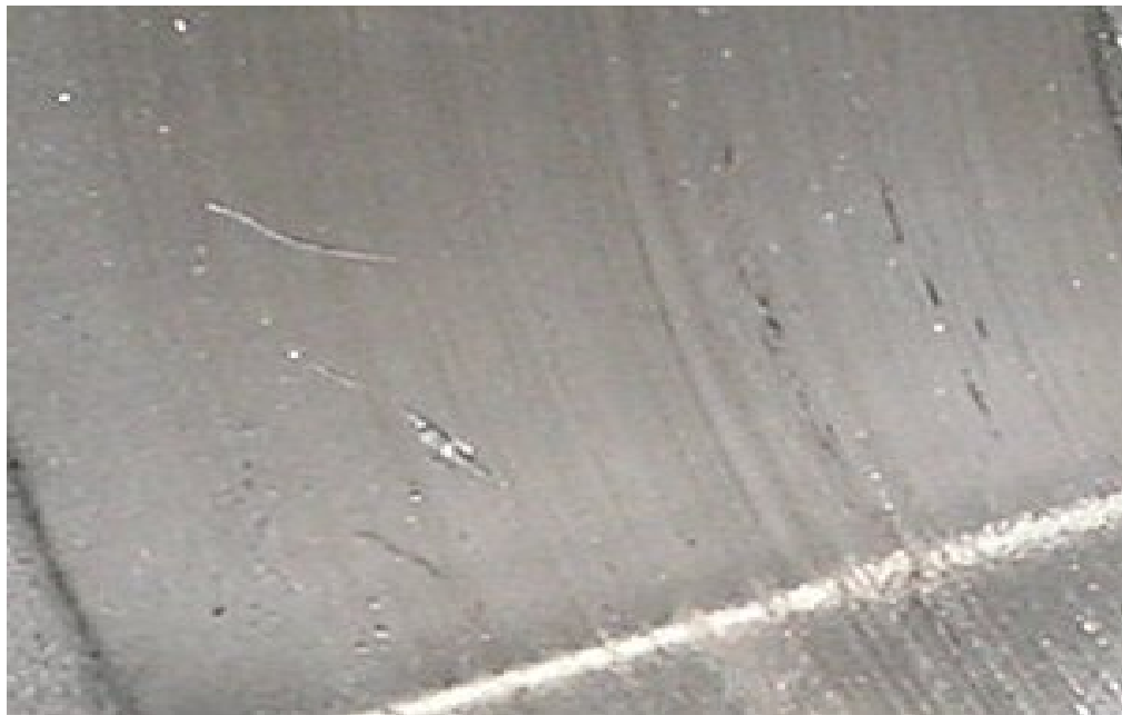
Figure 3: Another interior area of a knife-cutter after grinding printed circuit board. Note smeared material and nicks and scratches.
