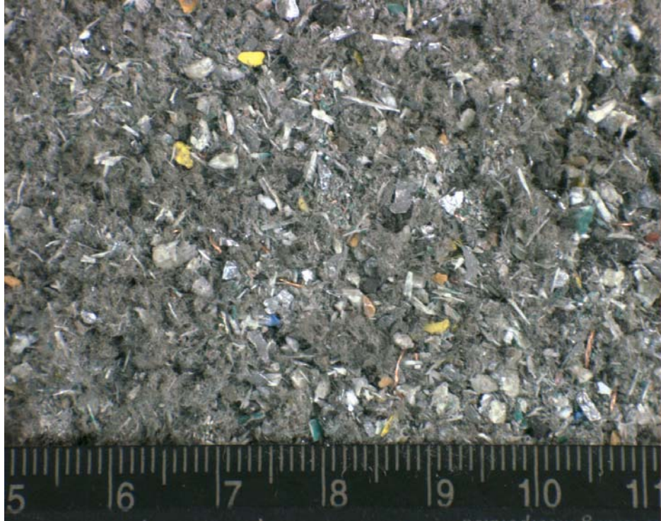
Figure 7: Close up of ground circuit board. Note wires and bits of components. Is this homogeneous?
