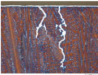
Turbine blade casting defect, outlined by a diffused chromium coating
