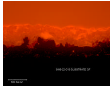
Figure 4: Plasma TBC-tested button with EC 2214 showing fluorescent epoxy from tensile adhesive in coating porosity-both bright field (a) and fluorescent filter (b).
