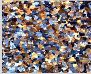
Commercially pure titanium (CPT) etched using dilute hydrofluoric acid and viewed under polarized light.
