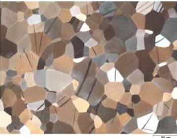
"Commercially pure titanium (CPT) etched using a dilute hydrofluoric acid solution and viewed under polarized light. CPT is commonly used for medical implants due to its light weight, high strength, bio-compatibility, and corrosion resistance."
