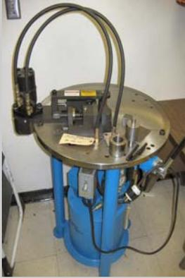
IMR Test Labs – Charleston recently purchased a new Hydraulic Bend Tester. Bend testing determines the ductility or the strength of a material by bending the material over a given radius. Following the bend, the sample is inspected for surface cracks. This provides insight into the modulus of elasticity and the bending strength of a material. With this new equipment we can test a wider variety of materials on site. This will better serve our existing customers and hopefully attract new ones.
