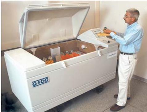
In the past 12 months IMR has acquired several major pieces of equipment to help us better serve our clients. (Clockwise from bottom left) Jody Russell, Lead Specialist-ESS & Electrical Testing, with Q-Fog Cyclic Corrosion Chamber; Fred Niggli, Machine Shop Preparation, with Struers Exotom-150 Chop Saw; Stan DeForest, Nonmetallics Manager, with Wabash 25 Ton Hydraulic Molding Press; Otto Roser, ESS/Product Test Specialist, with CM Rapid Temp Furnaces; a look inside the furnace at 2100°F.
