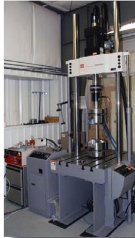
*Our New 55 kip MTS Fatigue Frame with T-Slot Table for Large Samples*
