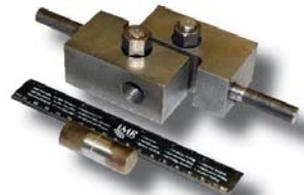
*Coating Shear Fatigue Fixture*
