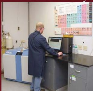
*Lead Chemist Brian Wackowicz Analyzing a Glass Sample on Ithaca's New XRF*
